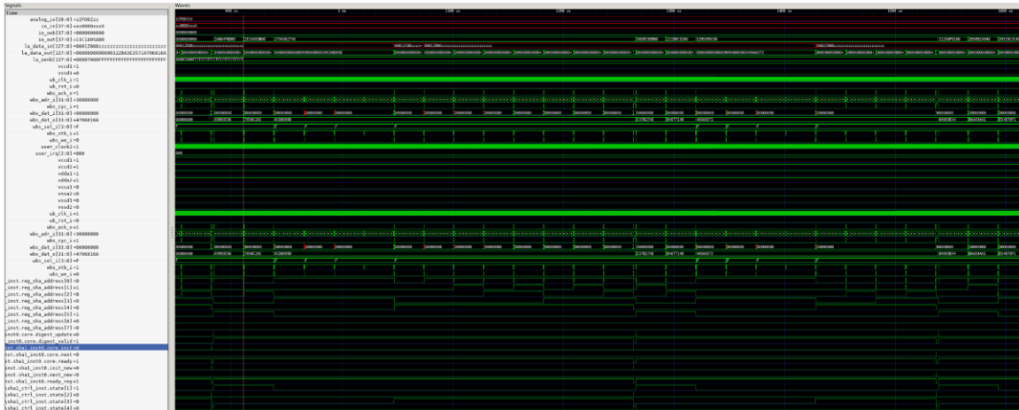
Figure 21. sha_top_test2 GL simulation showing all correct outputs (digests) using “abc” and “abcbcdcedefdefgefghghighijhijkijklklmklmnlmnomnopq” as input.
